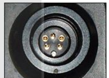
NIKONOS type 5 pin electrical sync connector and NIKONOS V with INON Z-22 strobe
